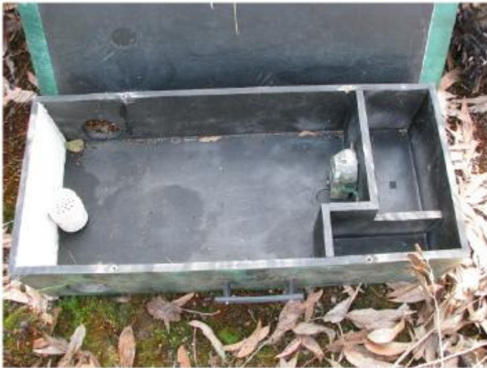
Interior of camera box. The bait holder is at the left.
